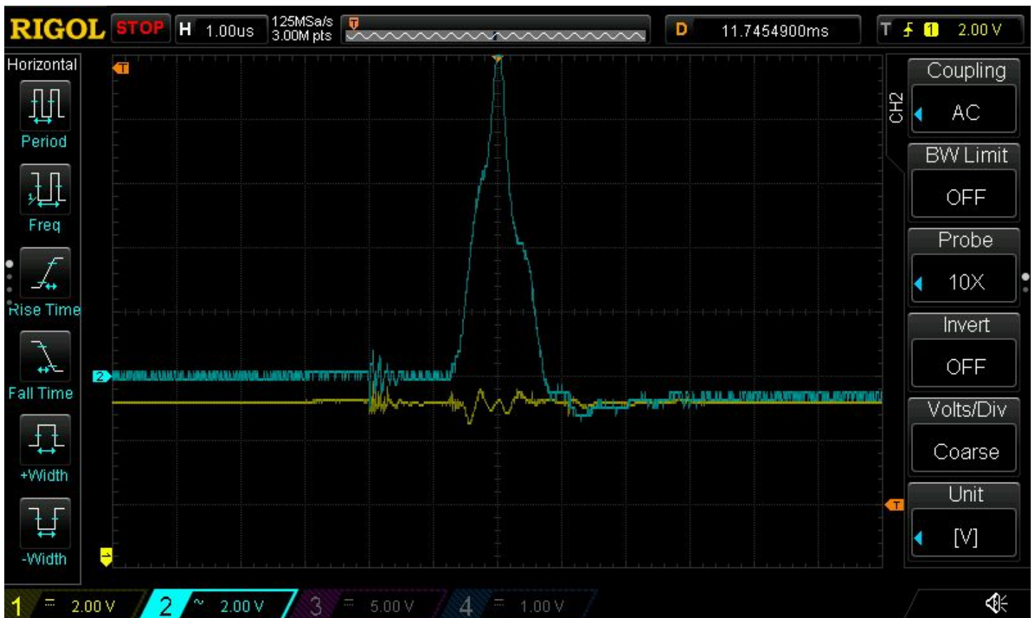
Figure 7. - Voltage spike on +38V auxiliary before repair, 10V peak.
