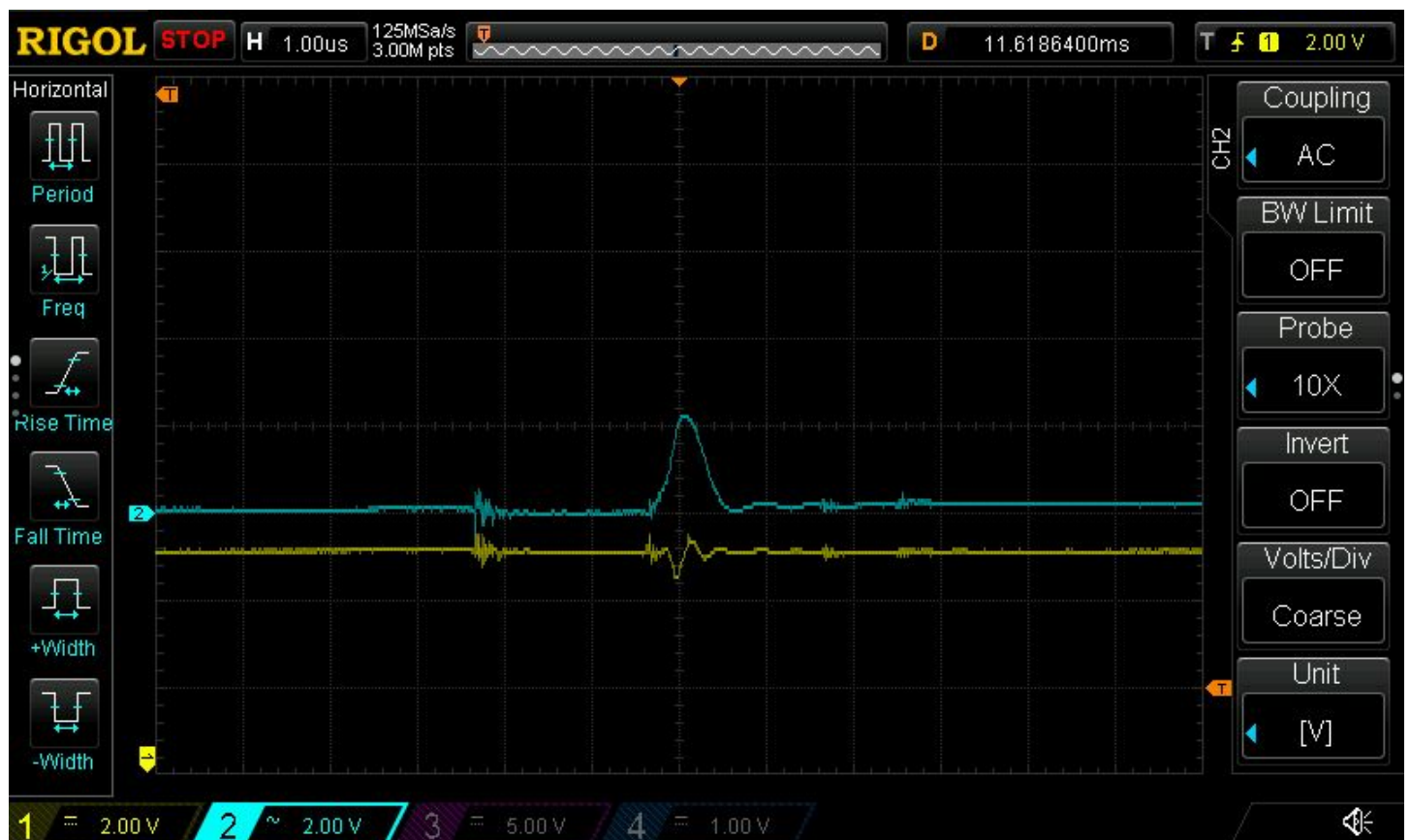
Figure 9. – Voltage spike on +38V auxiliary after repair, 2Vpeak.
